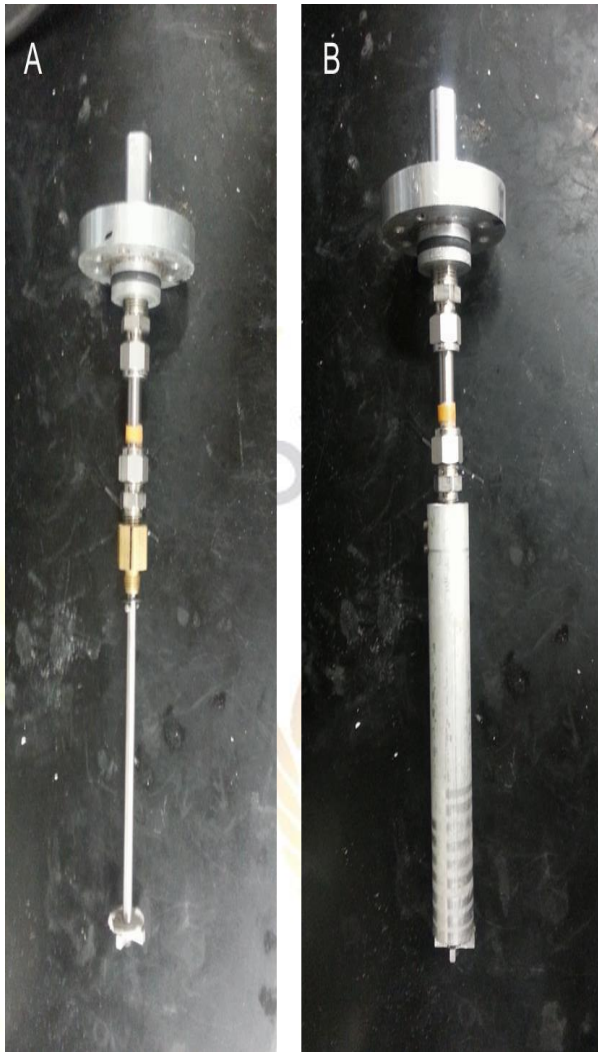
Figure 2 Photos of rotating mesh hopper assembly. Shown without (A) and with (B) concentric aluminum hopper insert that contains powder.
